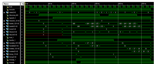
Fig. 3. Simulation result for 4-beat Incremental Burst Transfer Between Master-3 And Slave-1
