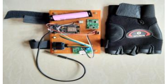
Fig. 3. Hardware model of heart disease predictor
