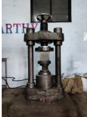
Fig. 7. Specimen placed on CTM
