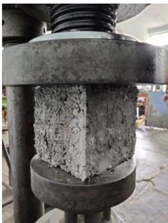
Fig. 9. Failure/breakdown of specimen
