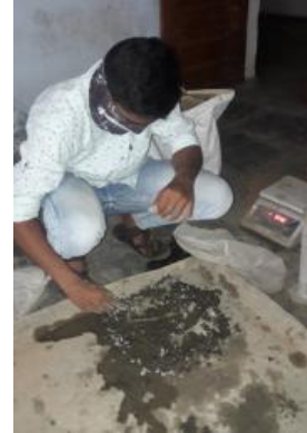
Fig. 5. Mixing of concrete
