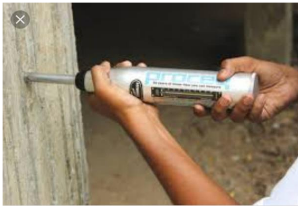
Fig. 2. Rebound hammer test
