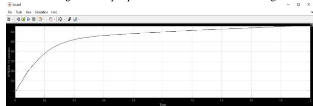
Fig. 13. PMSM load speed wave form in rad/sec (soft switching)
