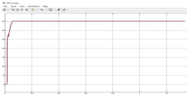
Fig. 11. Output voltage wave form of soft switching
