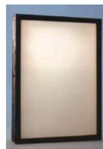
Fig. 4. Glass sample with black edging & aerogel-filled glazing cavity [4]
