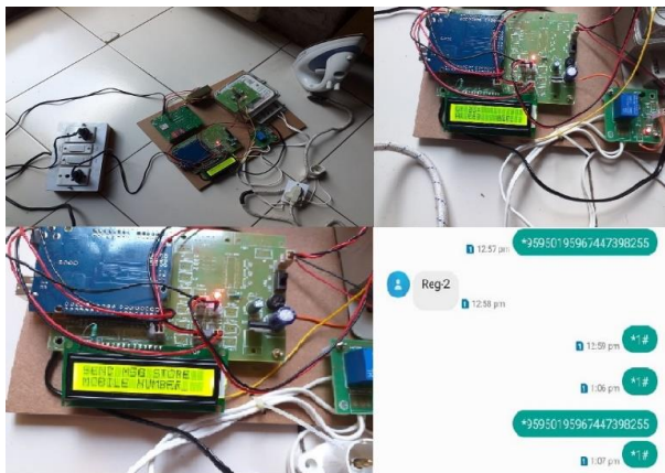
Fig. 10. Prototype arrangement and SMS received at consumer's mobile
