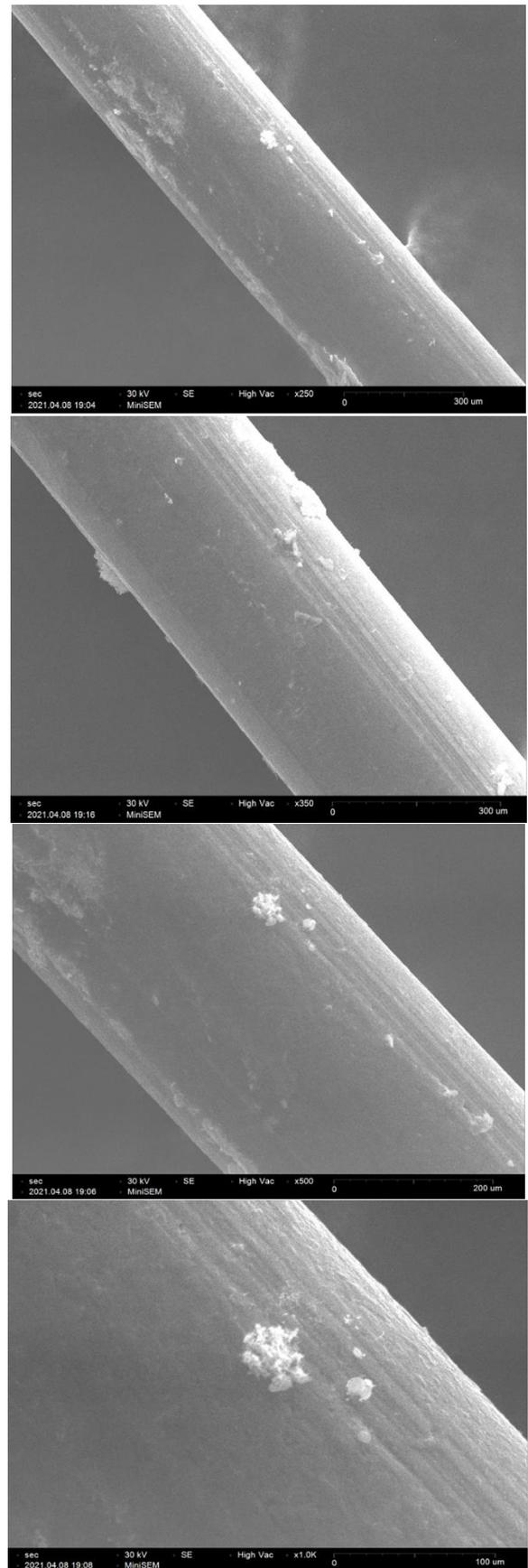
Fig. 13. Graphene (0.1% conc.) wire at 250X, 350X, 500X and 1000X magnifications
