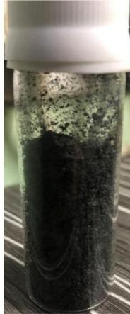
Fig. 1. Functionalized Graphene nanoplatelets
