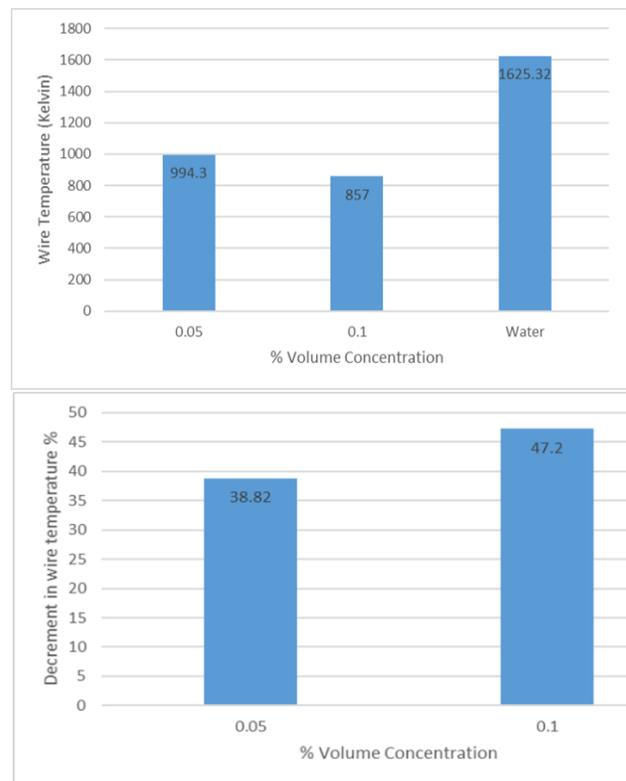
Fig. 11. Wire Temperature variation and Enhancement vs. Volume Conc.
