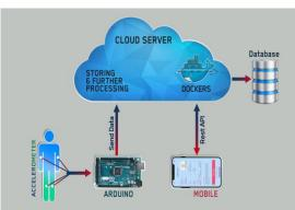
Fig 1. Architecture of the proposed system
