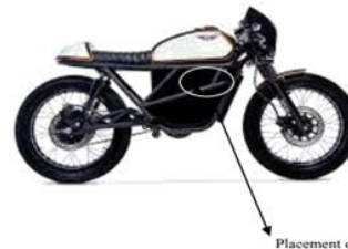
Fig. 1. Placement of designed circuit and battery
