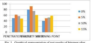
Fig. 1. Graphical representation of test results of bitumen after replacement of waste plastics
