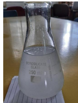
Fig. 4. 250ml of distilled water + 1gm CaO + 1gm Fly ash
