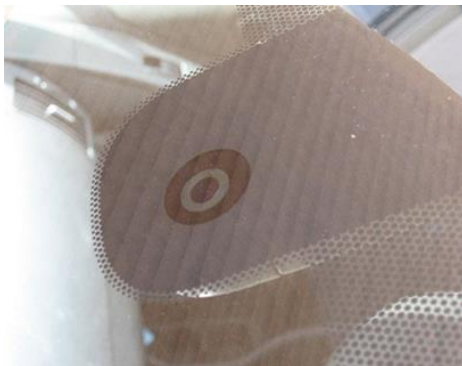
Fig. 4. Rain sensor on the windshield of a car
