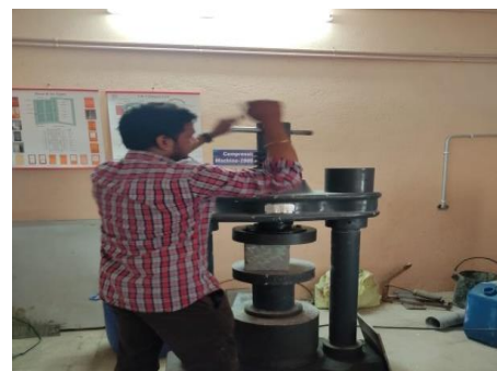
Fig. 6. Testing of cubes
