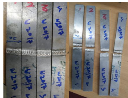
Fig. 3. Before and after tensile test
