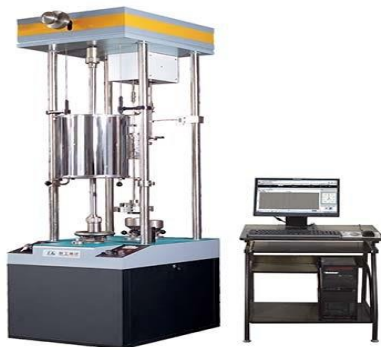
Fig. 3. Experimental setup of a creep tester
