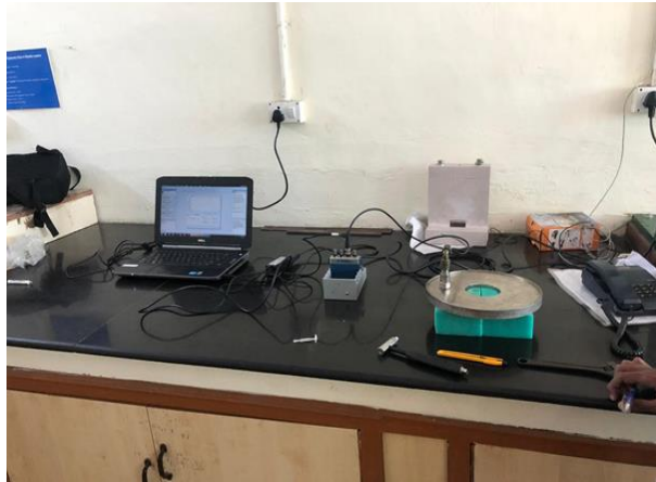
Fig. 2. Free vibration test using NI SIGNAL EXPRESS software
