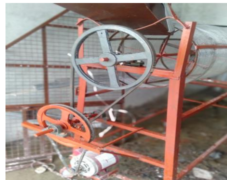
Fig. 14. Power supply system
