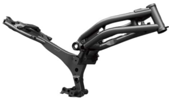
Fig. 7. Backbone chassis (left)
