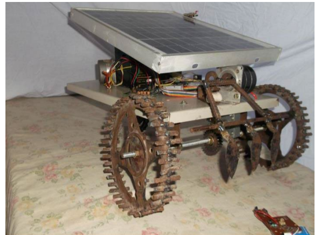
Fig. 2. Assembled prototype of the remote-control solar ploughing machine
