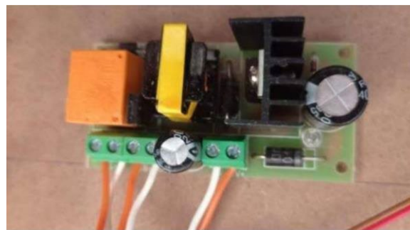
Fig. 5. Charge controller/solar regulator circuit board used to manage battery charging
