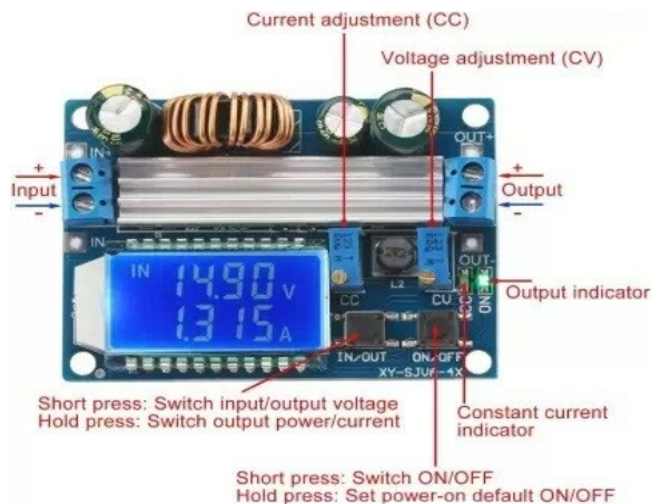
Fig. 8. DC-DC buck-boost converter module used to condition the combined source input
