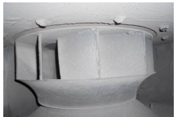
Fig. 4. Impeller before cleaning
