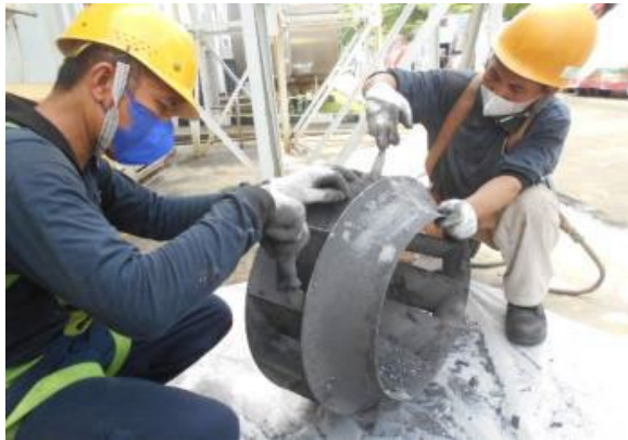
Fig. 5a. Cleaning impeller
