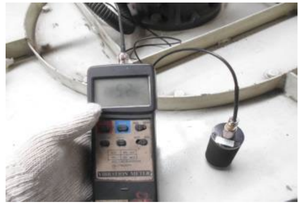
Fig. 3c. Initial vibration check (axial)
