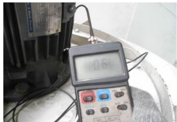
Fig. 7a. Final vibration check (horizontal)
