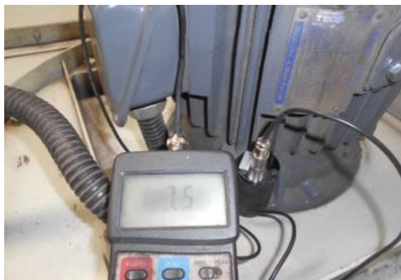
Fig. 3b. Initial vibration check (vertical)
