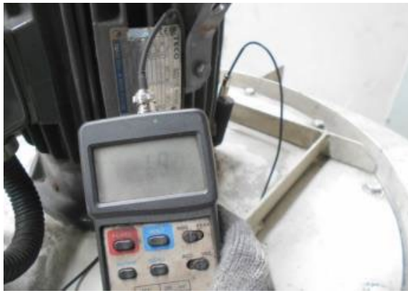
Fig. 7b. Final vibration check (vertical)
