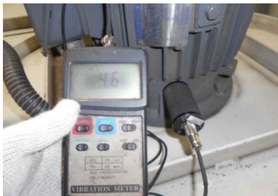
Fig. 3a. Initial vibration check (horizontal)
