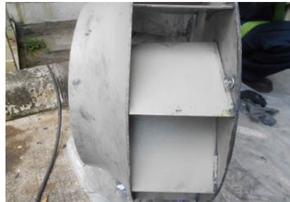
Fig. 7. Apply 5g weight
