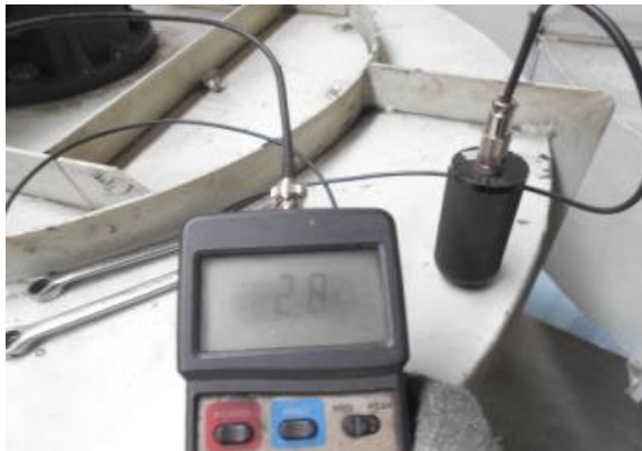
Fig. 7c. Final vibration check (axial)
