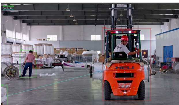
Fig. 2. Real-time perception output showing object detection, tracking, and distance-based safety estimation between human workers and industrial vehicles
