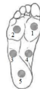
Fig. 3. Placement of five FSR sensors on the smart sock
