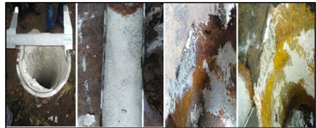
Fig. 2. Acid Pipe line examination: Thickness analysis, Colors test etc.
