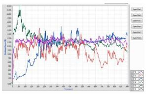
Fig. 8. Frictional force at 2000rpm
