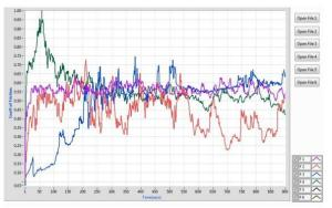
Fig. 10. Coefficient of friction at 2000rpm
