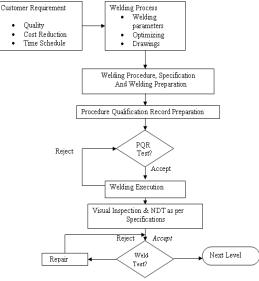
Fig. 3. Welding process flow chart
