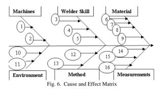
From the Matrix, 1. Equipments, 2. Tools, 3. Skill, 4. Training, 5. Qualification, 6. Electrodes, 7. Filer wires, 8. Filers, 9. Base & Filler defects, 10. Electrodes Storage Environment, 11. Base metal storage Environment, 12. Drawings and Specifications, 13. Weld matrix, 14. NDT 15. Non NDT, 16. Visual Inspection.
