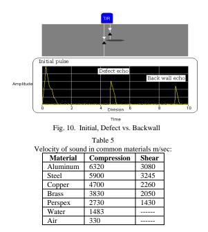
The weld shall be examined manually by pulse echo technique using shear wave probe and compression wave probe. Probe size and frequency for angle probe should be 8 mm\*9 mm crystal size and 2 MHZ to 5 MHZ, while normal probe size
