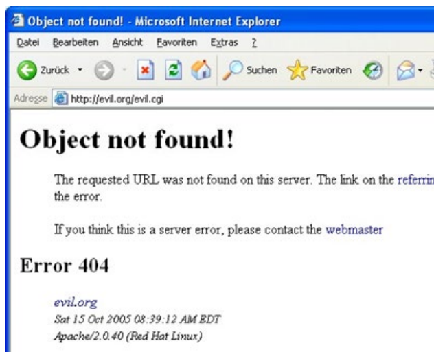
Fig. 5. Successful form-redirection attack to a non-existing URL
