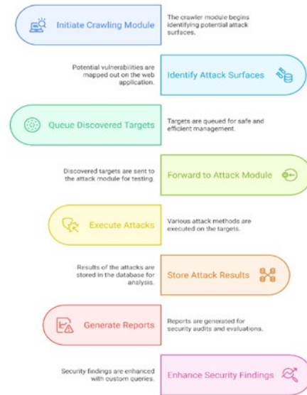
Fig. 3. XploitGuard attacking architecture
