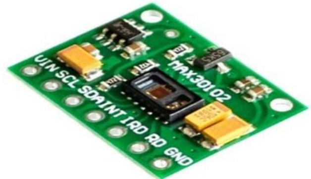
Fig. 4. MAX30100 SP02 sensor
