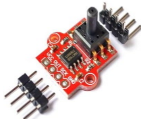
Fig. 8. HX710B pressure sensor
