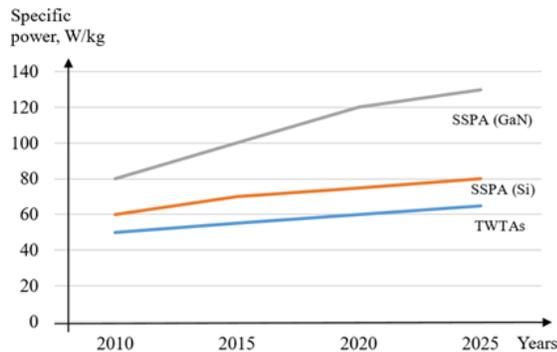
Fig. 2. Increase in Specific Power of Amplifiers (W/kg) [5], [14]
