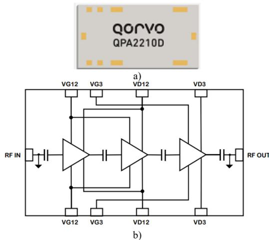
Fig. 1. Solid-State amplifier QPA2210D: a) External view, b) Block diagram
