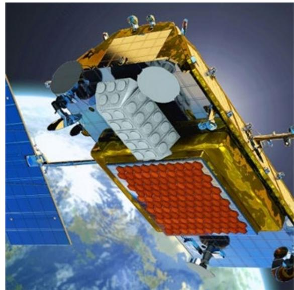
Fig. 4. View of the phased array antenna of the Iridium NEXT satellite
