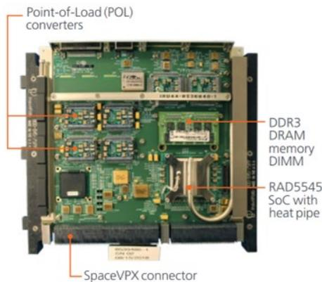
Fig. 3. GaAs processor RAD5545 [6]
