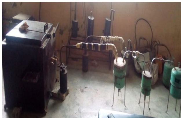
Fig. 1. Pyrolysis equipment setup (Renewable energy lab. LAUTECH)
