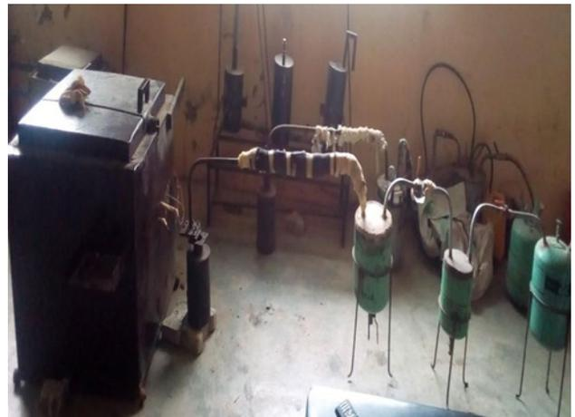
Fig. 1. Pyrolysis equipment setup
