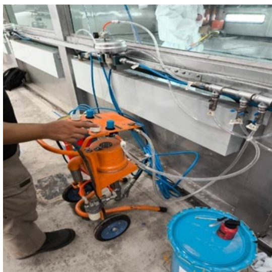
Fig. 10. Air-assist airless gun setting
