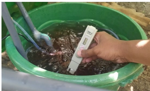
Fig. 7. Nutrient content and water volume measurements were conducted periodically throughout the cultivation process to achieve optimal nutrient levels and normal water volume
