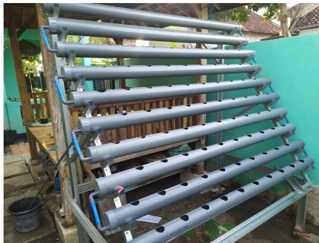
Fig. 2. Implementation of the DFT hydroponic system model with 100 planting holes (front view)
