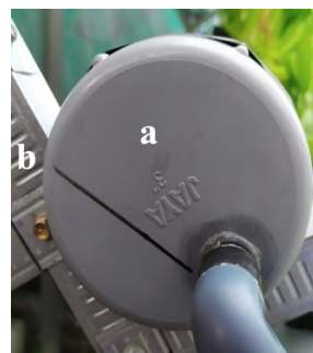
Fig. 5. The mechanism for adjustable caps to control the height of the nutrient water flow includes: (a) a 3-inch diameter pipe cap, and (b) 4x4 lightweight steel hollow material used as a support for the planting pipes
