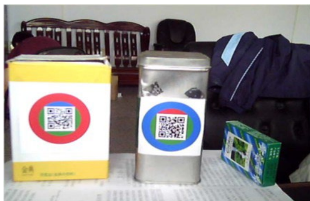
Fig. 2. Example of visual cue to aid QR code detection (reproduced from [9] with permission)
