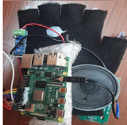
Fig. 5. Integration of Raspberry Pi, Arduino Nano, LCD screen, ultrasonic sensor, and gyroscope for a GestureSpeak
