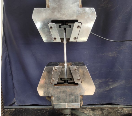
Fig. 3. Specimen mounted in an AFUTM device
