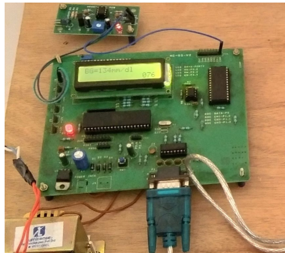
Fig. 8. Prototype of a noninvasive glucose monitoring device using NIR
