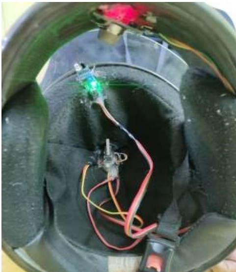
Fig. 9. Bottom view of helmet part displaying alcohol sensor, switch, eye blink sensor
