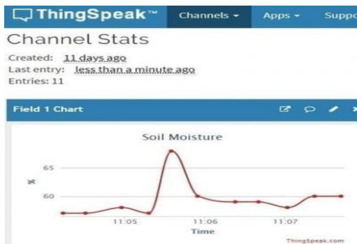
Fig. 4. Soil Moisture sensor value represented in graph on ThingSpeak
