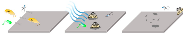
Fig. 2. Working process of fouling release coating Left to right: Organisms settling, Hydrodynamic shear force and Removal of the organism [21]
