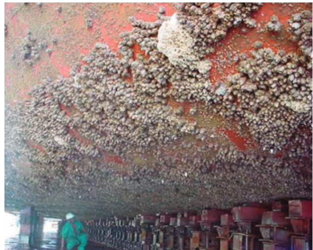
Fig. 1. Extensive Biofouling in the hull of a ship [14]
