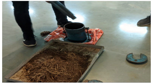
Fig. 12. Compacting of soil in 3 layers
