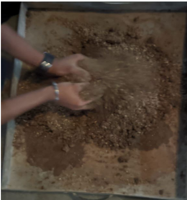
Fig. 10. Mixing of dry soil (160ml water)
