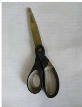
Fig. 5. Scissor used as tool for spatter creation
