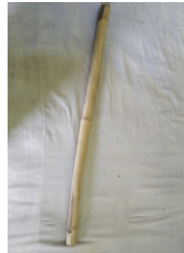
Fig. 7. Wooden log used as tool for spatter creation
