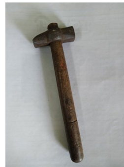
Fig. 1. Hammer used as a tool for spatter creation
