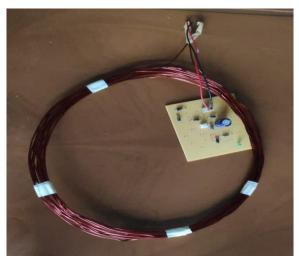
Fig. 4. Receiver coil of WPT
