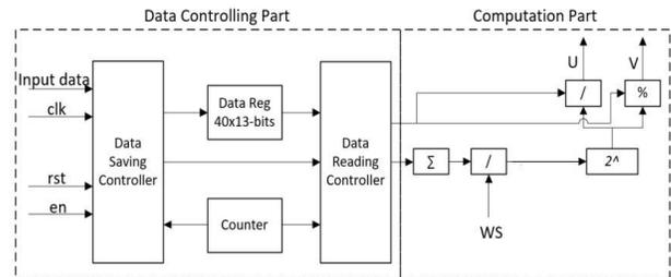
Fig. 5. Block diagram for Golomb rice coding
