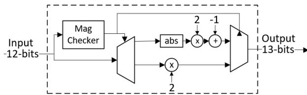
Fig. 4. Block diagram of error predictor
