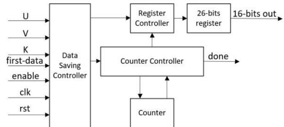
Fig. 6. Block diagram of packaging module
