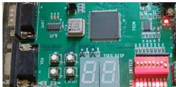
Fig. 12(c). Output obtained when the select line is 11
