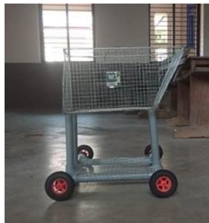
Fig. 3. Complete assembled figure of self-driving cart
