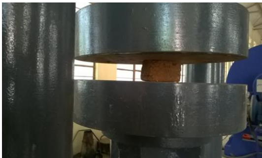
Fig. 1. Compression testing set up
