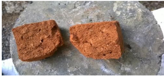
Fig. 4. Inner face of broken brick
