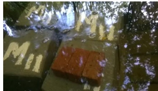
Fig. 2. Immersion and weighing of brick specimen
