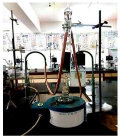
Fig. 4. Soxhlet apparatus for methanolic extraction
