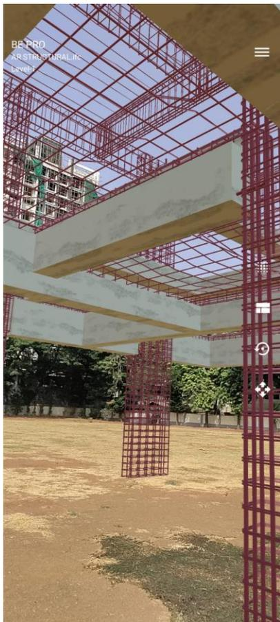
Fig. 19. Reinforcement Detailing in AR
