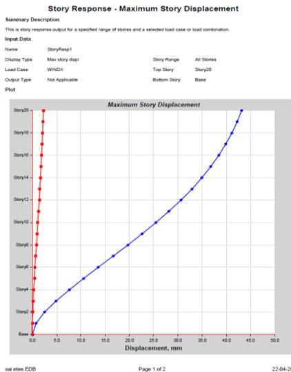
Fig. 5. Storey displacement (Wind X)
