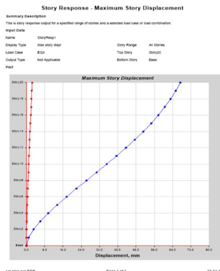
Fig. 6. Storey displacement (EQ X)
